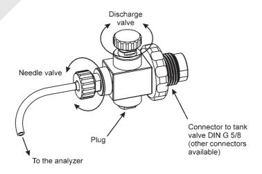
The analyzer switches into the helium and oxygen measuring mode upon activation, so there is no need for you to set up anything. Open the valve on the bottle to let the gas flow in. The gas composition is displayed after approximately 5 - 10 seconds. If the pressure inside the bottle is distinctly lower than 200 bars, the gas flow through the sampler will be slower and the measuring result will take somewhat longer to determine.
